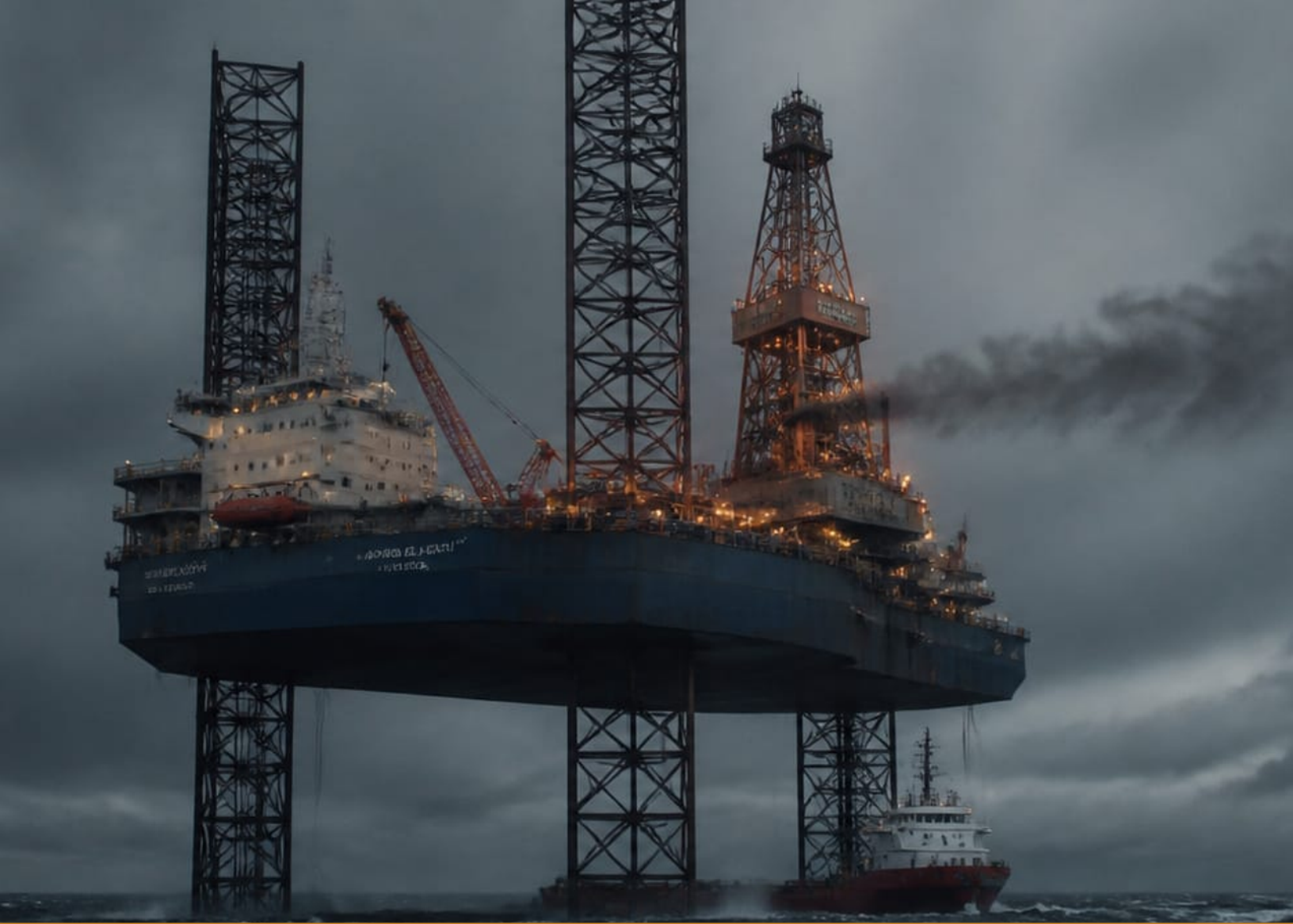
Jack-Up Drilling Rig — North Sea Self-elevating platform standing on the seabed in open ocean
