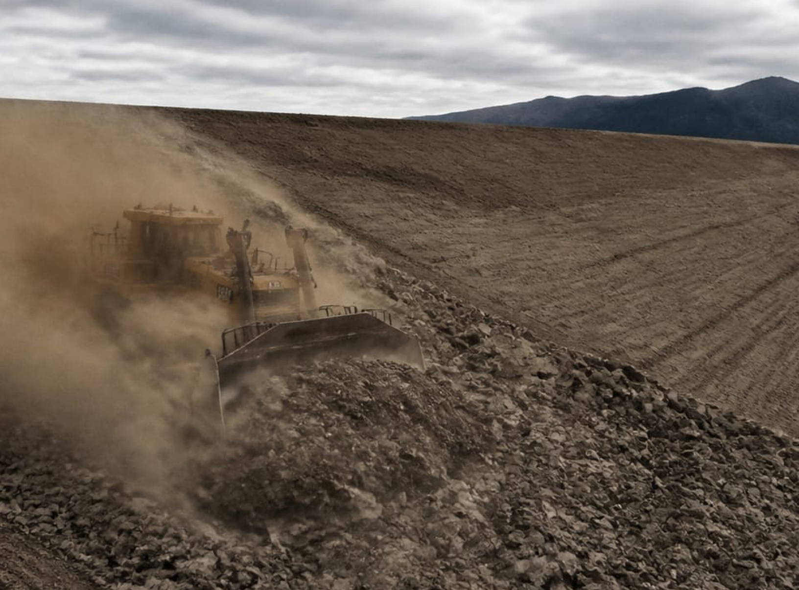
CAT D11 Bulldozer Largest production bulldozer · 850 horsepower
