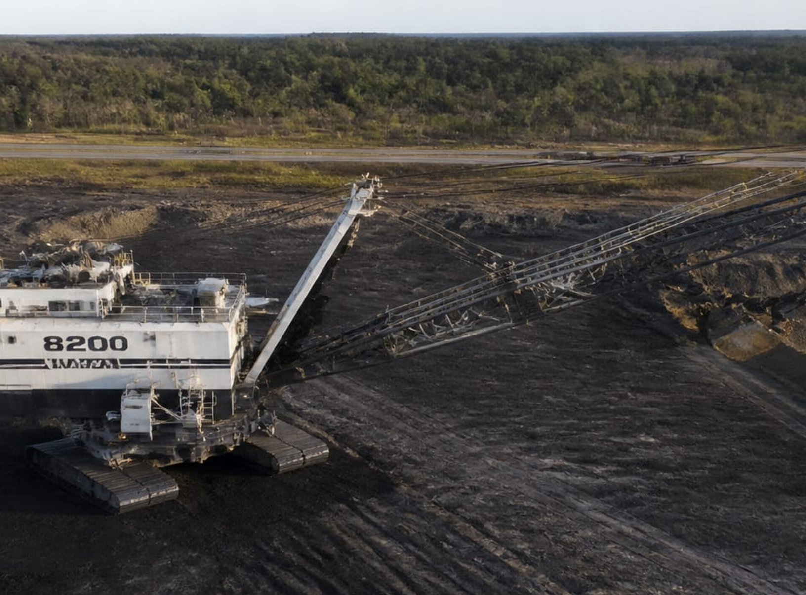
Marion 8200 Walking Dragline Coal mining dragline · moves on giant steel shoes
