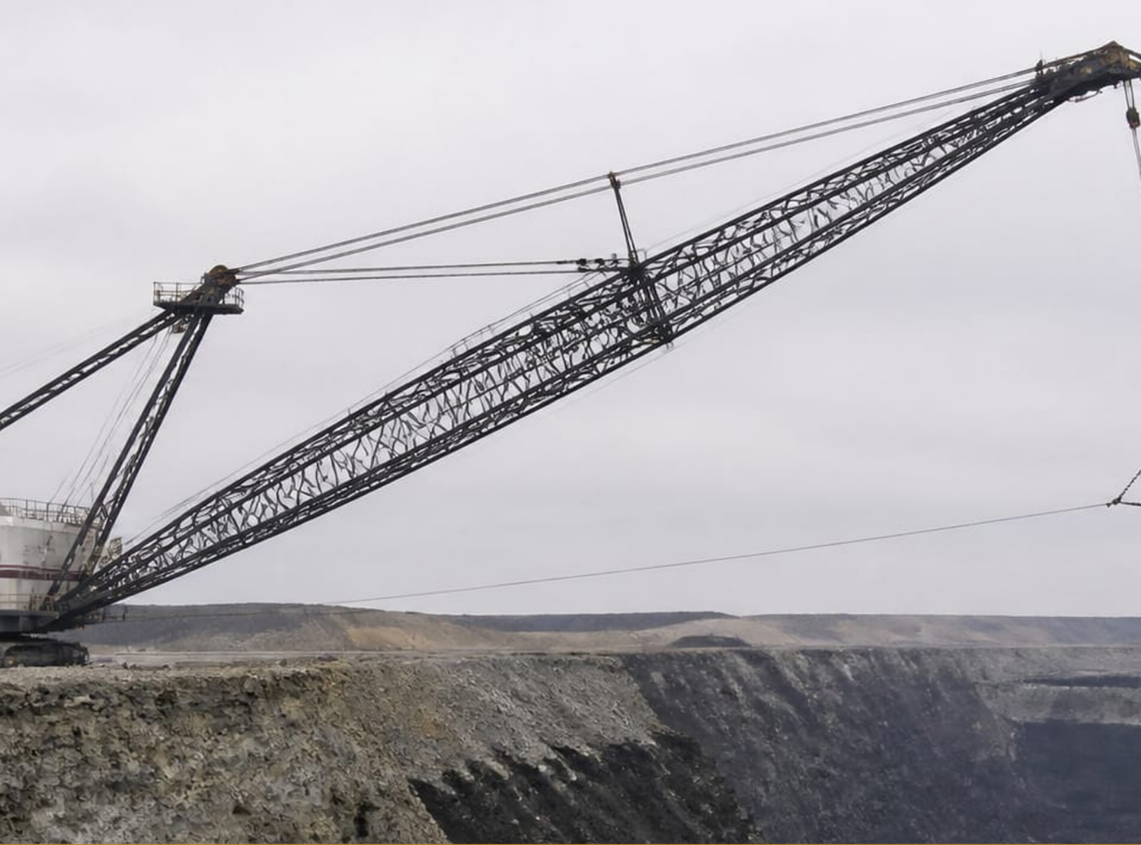
Bucyrus 8750 Dragline Crane Walking dragline · bucket holds 168 cubic metres
